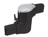
Syspend 180-Max Intermediate Joint joins two horizontal tubes together for a longer length. The arm can be rotated 300 degrees. Includes safety stop and maintenance-free bearings. Use of the intermediate joint reduces the system load rating capacity to 146 lb. (66 kg) at 3.3 ft. (1 m).
