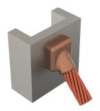
Heavy duty connections were originally developed to be used on reclaimed cable. The heavy duty connections use a larger size connection cavity in the mold and a larger size welding material than the equivalent standard duty connection.
