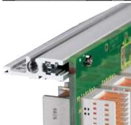
Rear horizontal rail for backplane mounting directly
