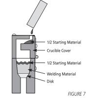
the mold cover, and pour the remainder in the opening of the mold cover. See Figure 7. Failure to comply may result in difficulty getting the reaction started and/or an unacceptable weld.
