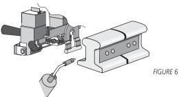
WARNING: Rebonding over the application of an earlier bond is only permissible in areas of minimal stress such as the head of the rail within the confines of the joint/splice bar! Remove the original bond by grinding down to a smooth layer of parent rail steel. The new bond can then be made in the same location as the previous bond. Failure to observe this may result in a rail break leading to property damage, injury or death to others.
