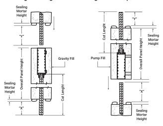
To Determine Typical Cut Length of Reinforcing Steel:
