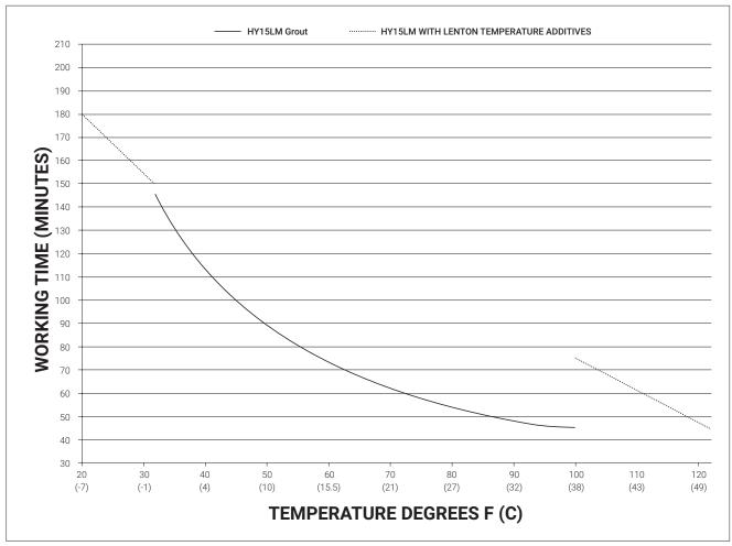
FIGURE 1: HY15LM - Approximate Working Time vs. Temperature
