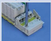
Remove the fuse by turning the fuse ejector 90 degrees using a 3/16" flat head screw driver (recommended.) Make sure the head of the screw driver is as large as the access point to prevent stripping the slot.
