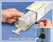
Replacement modules can be identified by the chart below or by the plastic strip on the side of the tray. A small flathead screw driver (above photo) will assist in removing the tripped module. Modules ship with a black key for use in dinrail bases. This key must be removed prior to installation into the TDX tray.
