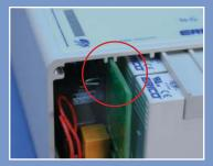
Make sure the green PCB board lines up with the slots as you slide the tray into the housing. Push tray firmly in to housing and replace base plate and screws. For models with a surge counter, the slot will start 1"(25.4mm) into the housing.
