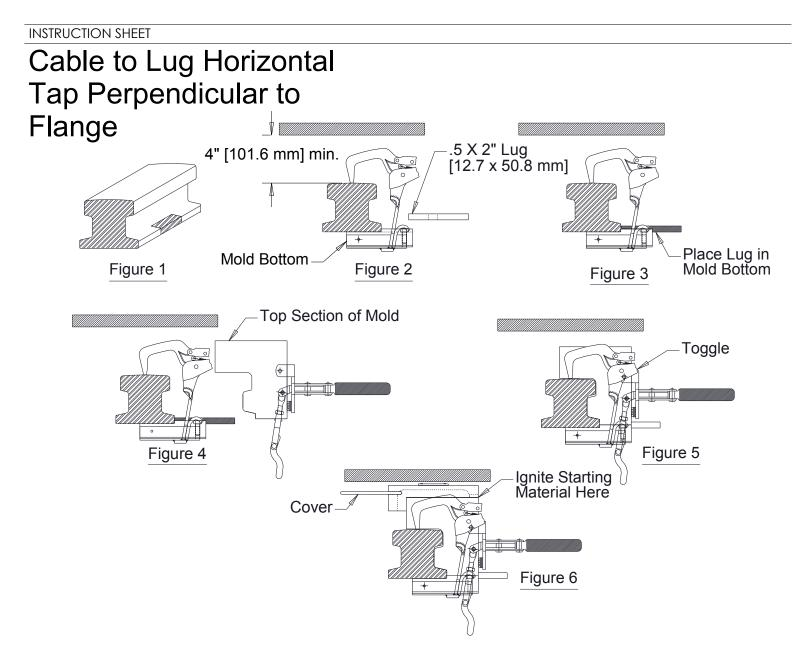
Prior to making a connection, read and follow the full instruction sheet IPRF, the full instruction sheet shipped with CADWELD<sup>®</sup> (IPX), and special instructions below.
