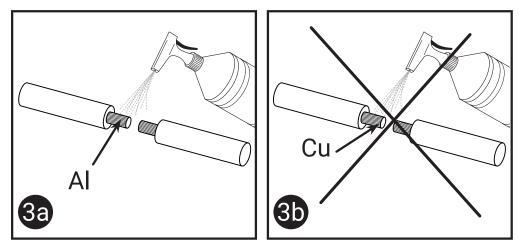
Immediately after cleaning aluminium conductors, use Cadweld Air Dry Flux T327A to prevent re-oxidation of the cleaned aluminium surface. There is no requirement to use Cadweld Air Dry Flux on copper conductors.
