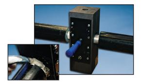
Cadweld molds are produced from graphite blocks and can be used for 50 or more welds. Molds for Al-Al and Al-Cu are different from Cu-Cu molds. Frames are needed in order to close the mold and hold it. Mold Sealer is required around the cable on the outside of the Cadweld mold to prevent leakage of molten weldmetal.
