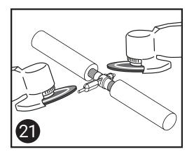
Remove risers and overflow at the Cadweld weld once material is solidified.
