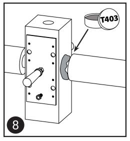
Apply (mold) sealer T403 between the mold and conductor to prevent leaking molten weld material.
