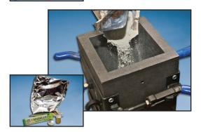
Cadweld welding material is a mixture of copper, aluminum and other ingredients. Each bag or container contains sufficient welding material for the specified connection. Cadweld welding material cannot ignite spontaneously. It can be handled and stored without danger. Adding starting material to the welding material is necessary to begin the exothermic reaction.
