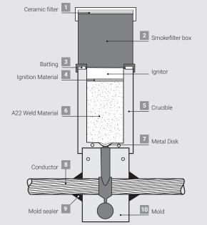
\*For Al-Cu connections, Copper must be tinned.
