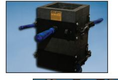
Cadweld crucibles are included in the mold design for smaller conductor diameters. Large welds will require a separate crucible in order to accept the required amount of welding material. Frames are needed in order to close the crucible and hold it.
