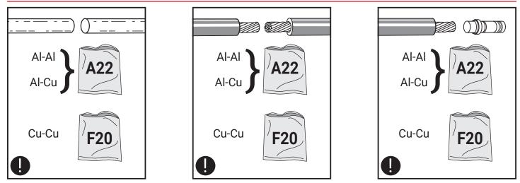
nVent offers welding material for different conductors. Please note that any Al-Cu or Al-Al connections require Cadweld A22 welding material. Cu-Cu connections will be processed with Cadweld F20 welding material.
