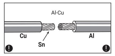
To provide a reliable connection between Al and Cu, the Cadweld welding process will require only tinned copper conductors.
