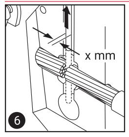
Please make sure that you maintain the correct "gap" between conductors inside the mold. This will allow the molten welding material to flow and connect the conductor. The number of the GAP Device shown on product overview pages 8 & 9 indicates the correct "gap".
