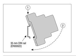
Surge Suppressor fixing clip to the bottom, ie label text the correct way up.
