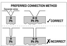
Where this is not possible due to layout or conductor sizing, use the "Non-preferred" "T" connection method as depicted on page 13. With this connection method, the "T" lead length should be kept as short as practicable (less than 100mm) and wires should be bundled together. The "T" conductor should be equal in size to the main conductor, up to a maximum of 6mm².
