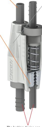
The locking device can accommodate wire rope at up to 90 degrees, allowing it to be positioned closer to the load than other locking devices on the market, hiding it from view and creating a much more aesthetically pleasing installation.
