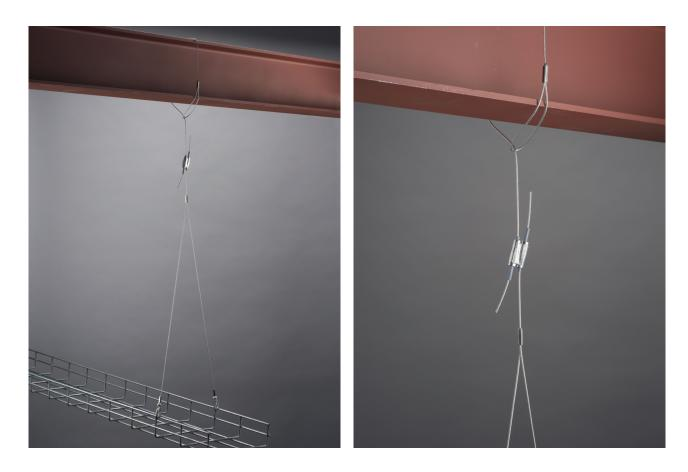
Splicing differs from normal cable hanging in that there is only one grip on each cable as opposed to the normal two grips. Because of this difference, the load rating is reduced, but maintains a safety factor of 5. See the table below for reduced working loads.
