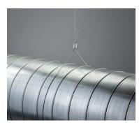
Speed Link attaches to structure differently depending on the end type. For fittings that attach at the load, the wire is looped around the structure and fed through the locking device. When end fittings attach at the structure, like the loop or toggle end fitting, the locking device is on the load side of the wire.
