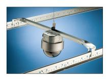
The SCMKC Security Camera Mounting Kit is easy to install by hand and is height adjustable to accommodate various electrical box depths.
