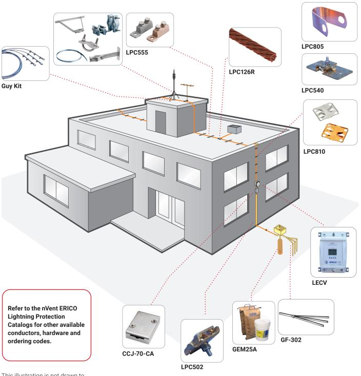
This illustration is not drawn to scale, nor does it portray an actual or typical application. It is designed to illustrate some of the major components of the nVent ERICO Lightning Protection System and their relationship with one another.
