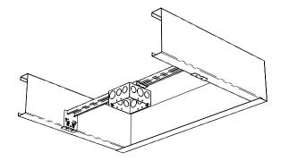
4. Position outlet box (outlet box not included) on bracket and secure with two (2) #12-24 screws provided.
