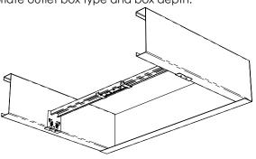
3. Secure bracket on either the flange or inside web of the wood or metal stud using the appropriate screw determined by the substrate (screws not included). The screw and stud shall have the appropriate strength to support the bracket. Two (2) screws required per side.
