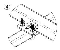
\*Min. Installation Torque: 60 in-lb [6.8 N-m]
