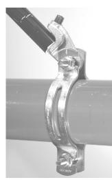
Insert brace pipe into brace clamp as far as possible. Tighten shear head set screw until head snaps off.
