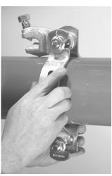
Rotate slotted stamped component over bolts. (Hardware does not have to be removed) \*Slot should face away from brace pipe.
