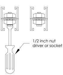
5. Tighten the STS until the strut assembly is secure.
