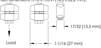
The STS may be inserted from either side of the strut.
