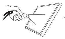
Flush the filter with warm water from the exhaust side to the intake side. Do not use caustics.
