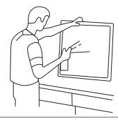
Recoat the filters with RP Super Filter Coat adhesive. When spraying filter do so from both sides for maximum concentration of adhesive.
