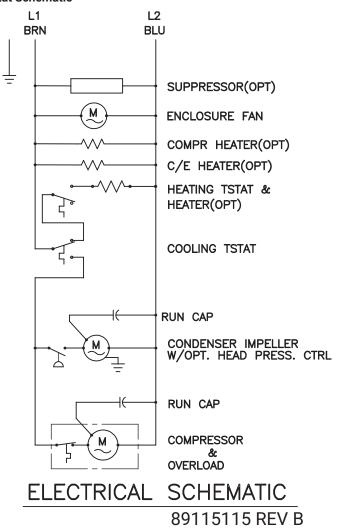
N21 with Remote Digital Controller, 115/230 V Wire Diagram
