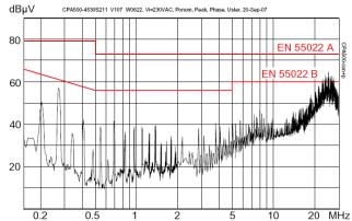
Typical disturbance voltage (peak) at the line input according to EN 55022, measured at  $V_{i nom}$  and  $I_{0 nom}$  CPA500
