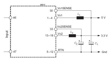
Output filter reducing the output ripple of Vo1 and Vo2
