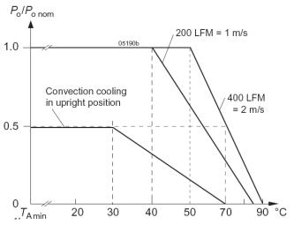
Output power versus temperature TA at Vinom (CPD/CPA250)
