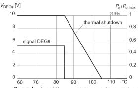
Degrade signal VDEG# versus case temperature Tc
