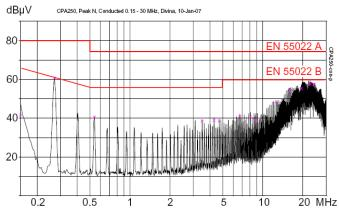
Typical disturbance voltage (peak) at the line input according to EN 55022, measured at  $V_{i nom}$  and  $l_{o nom}$  CPA250
