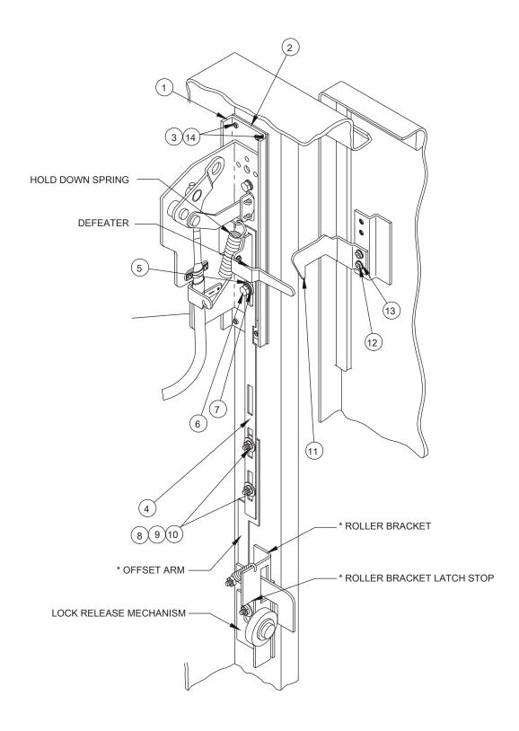
\* PARTS OF LOCK RELEASE MECHANISM
