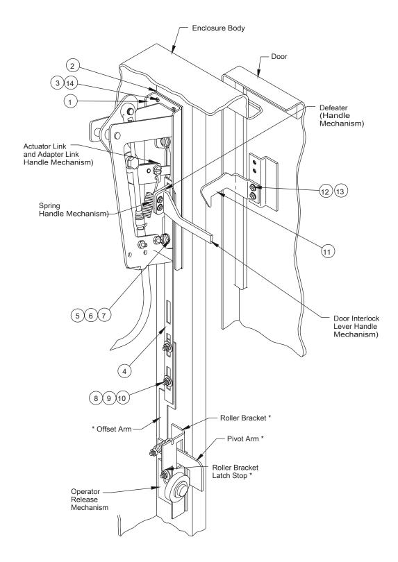
\* PARTS OF LOCK RELEASE MECHANISM
