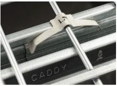
The nVent CADDY KBT Wire Basket Tray Clip is an easy-to-install time-saving solution for securely attaching wire basket tray to strut. Simply place the basket tray on top of the strut, position the KBT Tray Clip over the tray at the desired position, squeeze and slide it in place to finish the connection - it's that simple.
