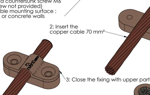
4: Screw this part to close the fixing with the 2 X M6 pozidriv countersunk head screw included at 5 Nm
