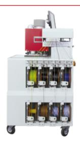
For flexibility on the fly, the magazine holds 8 types of wires
