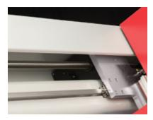
Ball screw spindles deliver precise holes and cutouts, as well as for low vibration, high tool life and a long service life
