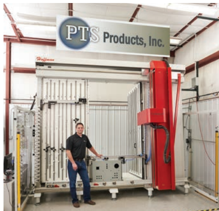
Paul Soberg, founder of Minnesota-based panel shop PTS Products, achieved higher quality and faster turnaround times by automating custom cutouts on its enclosures and back panels using the ModCenter.
