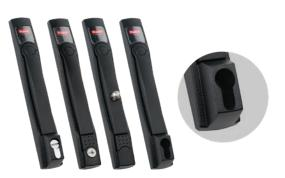
Flush Handles are optional for any solid, window or disconnect door greater than 600 mm in height, except Voice/Data and Colocation cabinets. They are ergonomically designed to provide style and function in a low profile. The handle is die-cast zinc finished with RAL 9005 textured black polyester powder paint. Provision to add your logo is included. Handle can be installed to rotate either clockwise or counterclockwise.
