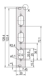
U-profile front panel with cutout for D-Sub connectors. Shieldable for textile EMC gasket.
