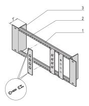
Module support is needed for assembly of partial width front panels with SUB-D-, ST type 3 or FDDI cut-outs, with or without strain relief rail.
