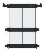
Doors at the end of the aisles are the third component that further isolates the hot air and cold air mixing in the computer room. In most computer rooms, hot exhaust airflow wraps around the sides of the racks at the end of an aisle. This results in significant mixing of the hot and cold air, and elevated inlet temperatures for the IT equipment in these racks.
