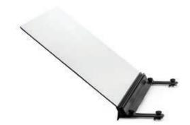
Typically installed on the top front edge of an IT rack in a cold aisle. The Rack Top Baffles extend from the front edge of the rack into the aisle, reducing the open area of the aisle and slightly pressurizing the cold aisle relative to surrounding areas. In addition, the Rack Top Baffles significantly reduce the recirculation of hot exhaust air from the rack equipment across the top of the rack and back into the front intake of the rack. These angled baffles cover 66% of the top of the aisle.
