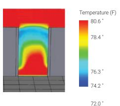
The CFD model shows significant recirculation from back to front on the end aisle racks. Hot exhaust air from the rear of the racks is wrapping around and being pulled into the equipment inlet on the front of the rack. The color red indicates temperatures exceed ASHRAE TC9.9 recommended temperature of 80.6 Deg F.
