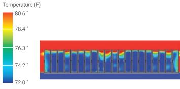
The CFD model shows significant recirculation of exhaust air over the tops of the racks. The color red indicates temperatures exceed ASHRAE TC9.9 recommended temperature of 80.6 Deg F.
