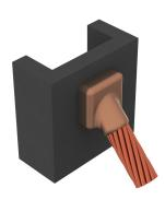
nVent ERICO Cadweld Cathodic Connections are the preferred method of exothermically welding cathodic protection anode leads to pipes (steel or cast iron), tanks, and other structures. Cathodic protection systems are designed to prevent galvanic corrosion along a pipeline or in various structures. nVent ERICO Cadweld Cathodic Connections use a special welding material alloy to minimize heat effect on the steel, which is especially important on thin wall and high stress pipes.
