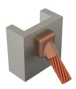
nVent ERICO Cadweld Cathodic Connections are the preferred method of exothermically welding cathodic protection anode leads to pipes (steel or cast iron), tanks, and other structures. Cathodic protection systems are designed to prevent galvanic corrosion along a pipeline or in various structures. nVent ERICO Cadweld Cathodic Connections use a special welding material alloy to minimize heat effect on the steel, which is especially important on thin wall and high stress pipes.
