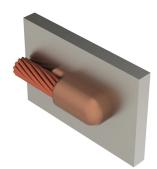
nVent ERICO Cadweld Cathodic Connections are the preferred method of exothermically welding cathodic protection anode leads to pipes (steel or cast iron), tanks, and other structures. Cathodic protection systems are designed to prevent galvanic corrosion along a pipeline or in various structures. nVent ERICO Cadweld Cathodic Connections use a special welding material alloy to minimize heat effect on the steel, which is especially important on thin wall and high stress pipes.
