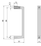
Slim Aluminium profile front handle, 9 mm. The assembly of the handle will be done from the rear side.
