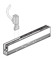
power connector for busbar achieves internal power distribution designed to reduce server complexity and providing a separable connection that ease assembly, inspection, and troubleshooting.
