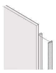
The textile EMC gaskets are inserted into a slot on the right hand side of the U-shaped front panels. The gaskets are glued to the front panel.
