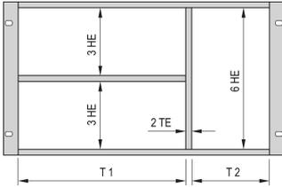
The combined mounting enable the option to split a 6 U high subrack or case in 2 x 3 U and 6 U sections. Different versions are available.
