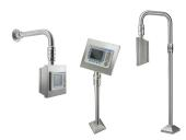
Specifically designed to support the Syspend Sanitary HMI Enclosure in sanitary washdown environments, particularly food and beverage manufacturing. The suspension system supports up to 90 lb. (40.8 kg) at 3.3 ft. (1 m). Its modular design with multiple tube lengths and bent tubes allows for application versatility. The entire system meets Type 4X and IP69K requirements for high pressure, high-temperature washdown applications.
