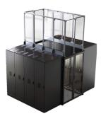
Works with a pod of cabinets surrounding a hot aisle. It is supported on top of the cabinets and channels the hot air exhausted from the server equipment housed inside the cabinets up to a ceiling plenum. This is used to completely separate the hot from cold air, drastically reducing data center energy costs.
