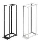
4-Post Open Frame Racks combine the mounting security of a cabinet with the accessibility of a rack. Used in communication data center and telecommunication room applications, these adjustable-depth racks support deeper, heavier network equipment and can be ganged with standard 2-post or other 4-post racks to expand existing systems.
