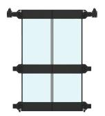
Designed for 48-inch (1200mm) wide aisles. Can also provide benefits for wider aisles. A 48-inch (1219 mm) wide version seals aisles from 46-inch (1168 mm) to 54-inch (1372 mm) and a 72-inch (1829 mm) wide version seals aisles from 70inch (1778 mm) to 78-inch (1981 mm). Custom solutions can also provide benefits for wider aisles.
