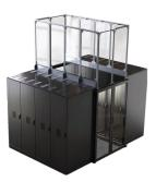
Works with a pod of cabinets surrounding a hot aisle. It is supported on top of the cabinets and channels the hot air exhausted from the server equipment housed inside the cabinets up to a ceiling plenum. This is used to completely separate the hot from cold air, drastically reducing data center energy costs.
