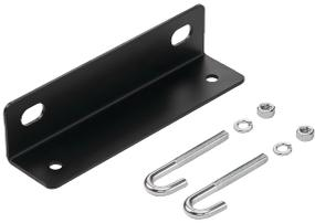
The Cable Runway Wall Angle Support provides support to ladder rack from a wall or other flat surface. It is made of 2-inch x 2-inch, 10ga painted or plated steel. The kit includes two J-bolts, nuts and screws.
