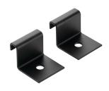
The Cable Runway Vertical Wall Bracket secures ladder rack sections to a wall or other flat surface. It features a U-shape hooking in the rails of the ladder rack with a 90 degree bend on the other end to mount to a perpendicular surface. It requires surface mounting hardware (not included).
