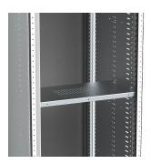
The galvanised steel shelf, MSCC, covers a partial depth of an enclosure and is ideal for equipment requiring strong fixation, such as heavy air circuit brakers. It leaves the rear of the enclosure accessible for easy installation and wiring.
