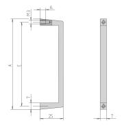
Slim Aluminium profile front handle, 7 mm. The assembly of the handle will be done from the rear side.
