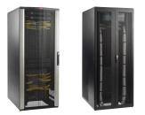
ProLine Network Switch cabinet is a pre-engineered solution for the thermal and cable management needs of large data center network core switches. It is designed to meet Cisco 6509, 6513, 7009 and 7018 Series network switch requirements in data centers with a hot aisle/cold aisle cabinet layout. (For other Cisco switch models, contact HOFFMAN for cabinet applications.) Cabinet provides for both patch cords and permanent link cables with support from vertical to horizontal transitions.
