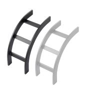
The Ladder Rack Curved Sections provide a vertical change in direction. They are made of 1-1/2 inch x 3/8 inch (38 mm x 8 mm) tubular steel with a painted or plated finish. Cross members are welded on the inside (inside bends) or outside (outside bends) of the section. They connect to straight section with butt-splice kits. They are also designed for category 5e, 6, 6A and fiber optic cable.
