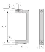
The handle can be assembled to a subrack or 19" front panel. Available with clear or black anodized surface. Handles will be bolted from the rear side.
