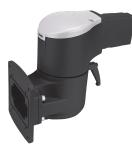
Syspend 180-Max Horizontal Panel Coupling mounts a horizontal tube to the back of an enclosure or screen using Video Electronics Standards Association (VESA) mounting. The coupling has mounting holes drilled for standard VESA 75 and 100 flange sizes. It enables the enclosure to rotate 300 degrees and can be locked into a given position. The horizontal panel coupling has a safety stop and maintenancefree bearings.
