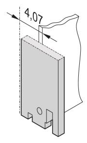
Front panel without or with SUB-D-, ST type 3- or FDDI cut-out.
